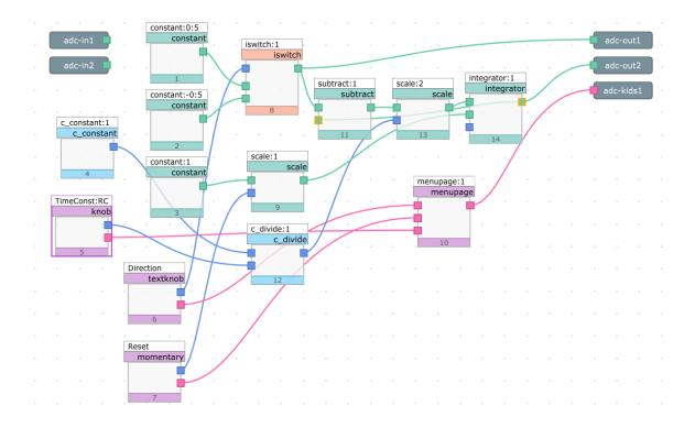
A signal (forcing function) can be substituted in place of blocks 8 and its predecessors (for implementation in an application). In the example above provides a step function that varies between -0.5 and +0.5. The top line below is the input, and the bottom line below is the output. The RC at the start is 1000, rising to 10,000, 32,000 and then 1, 100, 1000 and 10,000. At bar 23 and 41 the reset is pressed resetting the integrator to 0.
