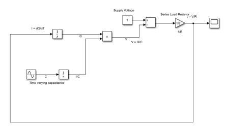
In our case, we will set the capacitance and load resistance as a variable, collect them by simplifying the block diagram to create a time constant (RC) and vary the voltage as the signal with a switch (0.5 and -0.5).
