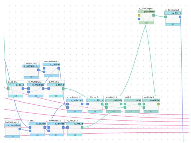
The Backstep operator or shift register is implemented by the 1 sample picodelay. The outputs 39 and 43 both give the envelope shape, 1 sample apart. Pick whichever one you want to feed the parameter you want mapped to the envelope.
